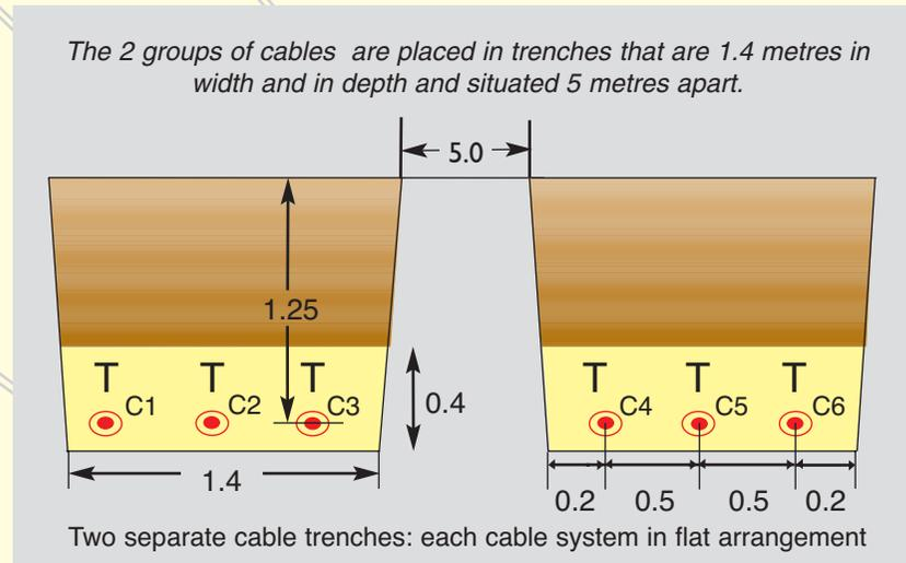
Modern Underground Cables with cross-linked polyethylene insulation (XLPE) are an alternative to the historically well proven technology of Overhead Lines. These Underground Cables are easy to install, easy to maintain and easy to repair. **Several Underground projects with lengths up to 210 km are under consideration in Europe at present.**
